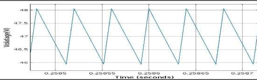
Fig.12. Load voltage ripple for boost converter
